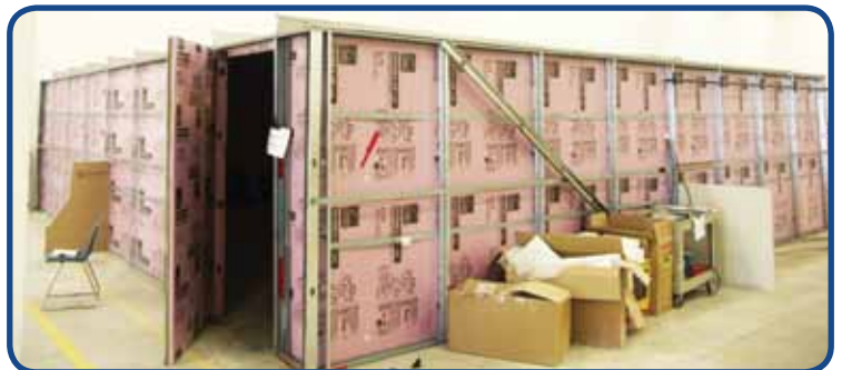
Photo: 1,000 square foot room (32'x32'x8') constructed for testing described in this report.
